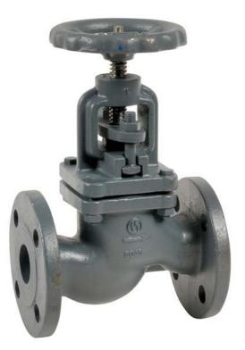
Size : DN 15 to DN 200 Ends : PN16 Flanges R.F. Min Temperature : - 10°C Max Temperature : + 120°C Max Pressure : 16 Bars Specifications : Rising rotating stem and handwheel Bolted bonnet and gland pack SS seat
