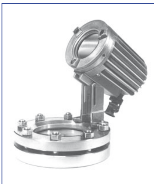
Complete assembly of sightglass fitting to DIN 28120, DN 125, PN 10, with glass disc of toughened sodium silicate to DIN 8902, fitted with CHEMLUX® sight glass slight fitting, type L20 deH Sch, tilting hinge fixation
