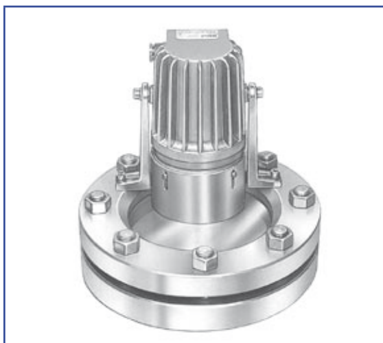
VETROLUX® illuminated sightglass unit, consisting of sightglass to DIN 28120, DN 150, PN 10, with mounted CHEMLUX® light fitting, type KEL 20 deH Sch B, 230 V, 20 W, EEx de IIC T4, Ex II 2 G + D, with anti-dazzle shield “B”, in version “view and light through one assembly”
