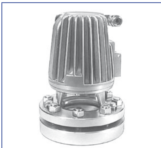
VETROLUX® illuminated sightglass unit, consisting of sightglass to DIN 28120, DN 80, PN 10, with mounted CHEMLUX® light fitting, type F 20dHNsp, 24 V, 20 W, EEx d IIC T5, Ex II 2 G + D
