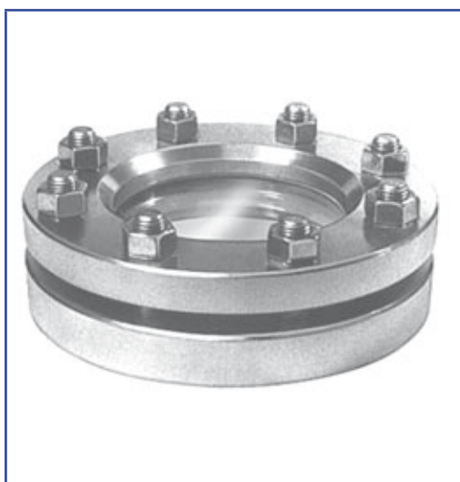
Complete assembly of sightglass fitting to DIN 28120, DN 100, PN 10 with glass disc of borosilicate to DIN 7080
