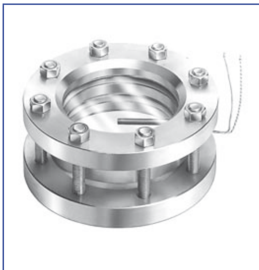
Double glazed sightglass similar to DIN 28120, DN 150, PN 16, with integrated heating element, 24 V, 50 W.
