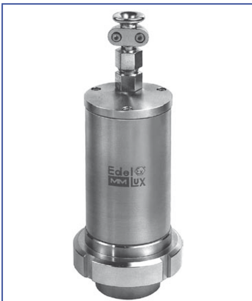
Sightglass light fitting type EdelEx 10 dH R50 K1, 10 W, 230 V, EEx d IIC T4, Ex II 2 G + D, with intermediate flange collar fixation "R", mounted onto a screwed sightglass similar to DIN 11851, PN 6, DN 50.
