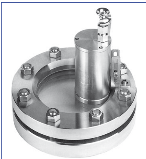
Sightglass light fitting type EdelEx 20 dH Sch K1, 20 W, 24 V, EEx d IIC T4, Ex II 2 G + D, mounted onto circular sightglass to DIN 28120, PN 10, DN 125.
