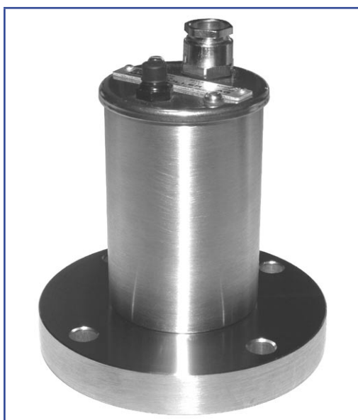
Sightglass light fitting type BKVLR 20 HDA, 20 W, 24 V, with built-in momentary push-button "D", on metal fused sightglass for aseptic flange connections to DIN 11864-2, DN 50
