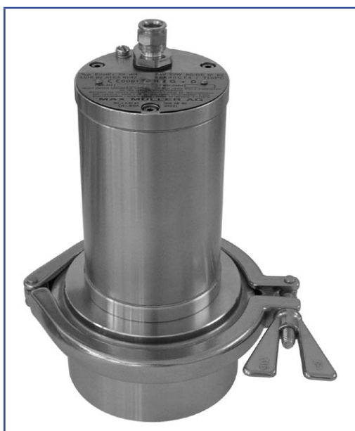
Sightglass light fitting, type EdelEx STERI-LINE 20 dH, 24 V, 20 W, EEx d IIC T4, Ex II 2 G + D, on metal fused sightglass, DN 100
