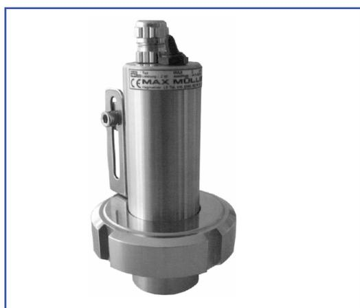
Micro LED light fitting, MVLR 2 LED E Sch1, 2 W, 24 V AC/DC, with integrated ON-OFF switch "E", mounted on VETROLUX screwed sightglass similar to DIN 11851, DN 32, PN 6
