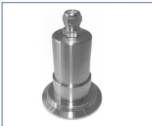
Micro LED light fitting, type MVLR 2 LED, 2 W, 24 V AC/DC, mounted on metal fused sightglass for Triclamp® fitting, DN 50, PN 16
