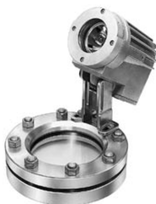
Type PEL 20 deH Sch, 230 V, 20 W, EEx de IIC T6, Ex II 2 G + D, mounted on circular sightglass to DIN 28120, DN 125, PN 10, in 1 port version
