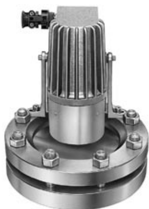
Type PEL 50 deH X2 B, 230 V, 50 W, EEx de IIC T4, Ex II 2 G+D, with anti-dazzle shield "B", on circular sightglass to DIN 28120, DN 150, PN 10, in version "view and light trough one assembly"
