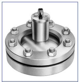
Sightglass light fitting type KVLR 20 HDW, 20 W, 24 V, with built-in momentary push-button "D", mounted with tilting hinge "Sch" on sightglass to DIN 28120, DN 100, PN 10, for application "view and light through one assembly".
