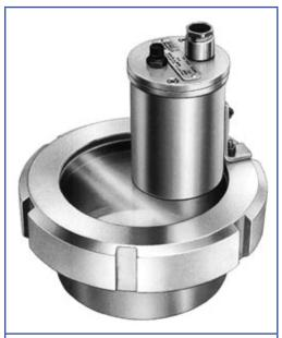
Sightglass light fitting type KVLR 50 HDW1, 50 W, 24 V, with built-in momentary push-button "D", mounted by bracket "W1" on screwed sightglass similar to DIN 11581, DN 100, PN 6, for application "view and light through one assembly".
