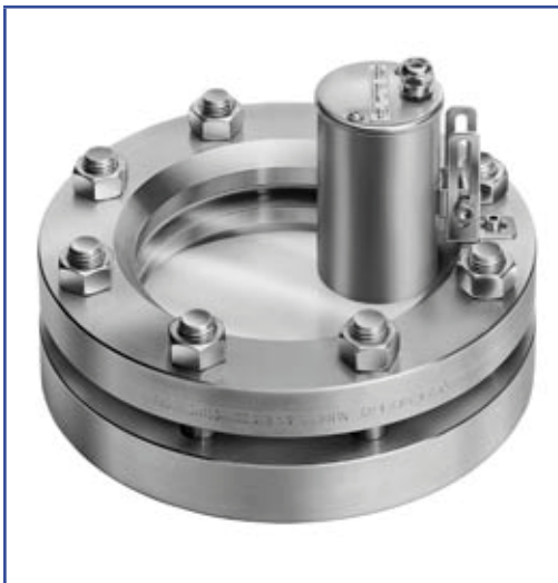
Sightglass light fitting type KLR 50 HSch, 50 W, 24 V, mounted with tilting hinge "Sch" on sightglass to DIN 28120, DN 100, PN 10, for application "view and light through one assembly".
