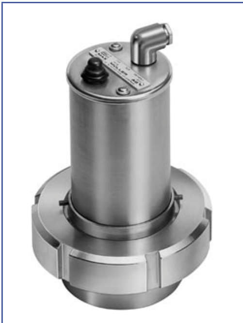
Sightglass light fitting type KLR 100 HD R80 K2, 100 W, 24 V, with built-in momentary push-button "D", mounted with flange collar "R 80" on screwed sightglass similar to DIN 11851, DN 80, PN 6.
