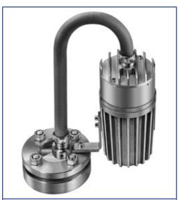
Fibre-optic lightpipe light fitting with built-in timer "U", type fibroLUX" 5035 W W2 U sp, EEx de IIC T3, Ex II 2 G + D, 35 W, 12 V DC, fixation of the light source by bracket "W", fixation of the lightpipe by universal support "W2" onto sightglass to DIN 28120, DN 40, PN 10
