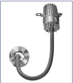
Fibre-optic lightpipe light fitting for use in hazardous areas with built-in timer "V", type fibroLUX® 5035 X1 W2 V, EEx de IIC T4, Ex II 2 G + D, 35 W, 230 V, fixation of the light source by fixation legs "X1", fixation of the lightpipe by universal support "W2" onto sightglass to DIN 28120, DN 40, PN 10
