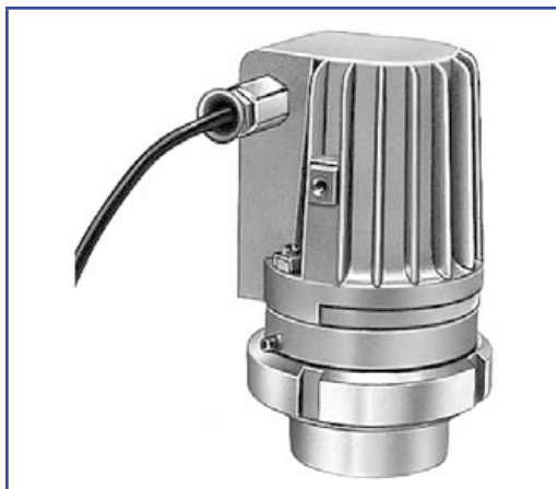
Hazardous area type FKEL 20 dH R, EEx d IIC T4, Ex II 2 G + D, 230 V, 20 W, on screwed sightglass similar to DIN 11851, DN 65, PN 6. Fixation with intermediate flange collar "R".
