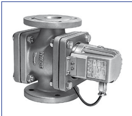
Hazardous area type FKEL 5 dH WM, EEx d IIC T6, Ex II 2 G + D, 230 V, 5 W, with opal glass "M", on pipeline flow indicator DN 50.
