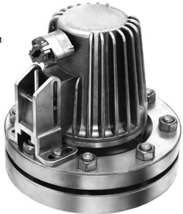
Type F 20 dHSchU, EEx d IIC T5, Ex II 2 G + D, halogen bulb, 230 V, 20 W, with built-in timer «U», mounted on sightglass to DIN 28120, DN 125, PN 10, with tilting hinge fixation "Sch"
