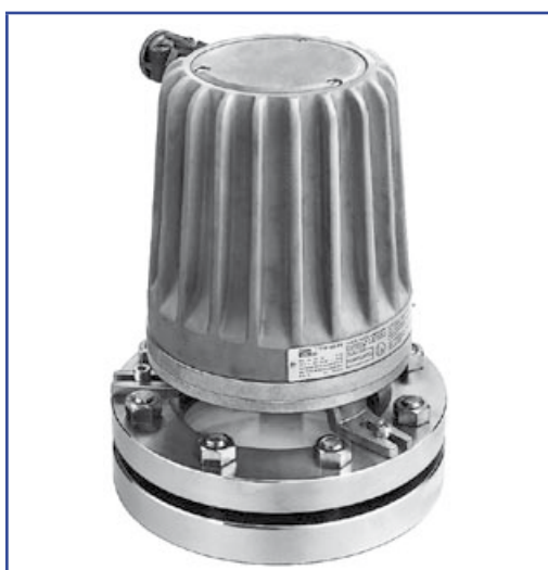
High performance sightglass light fitting type 100 deHN, 100 W, 24 V, EEx de IIC T4, Ex II 2 G + D, foot ring fixation on sightglass to DN 28120, PN 10, DN 125
