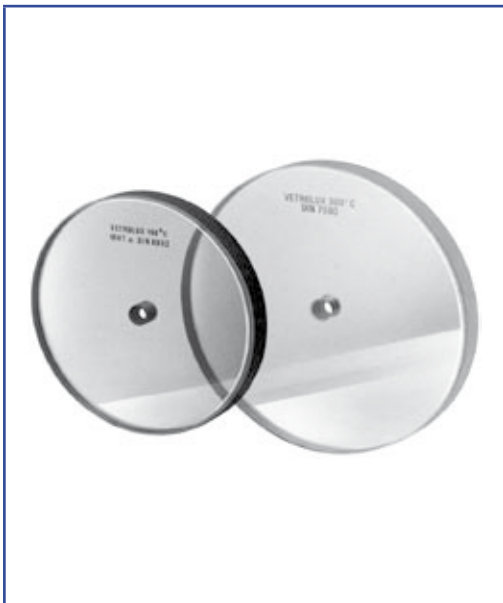
Sight glass discs similar to DIN 8902 or DIN 7080 with central bore \varnothing 10,5 mm to fit our wipers of the series W/WD
